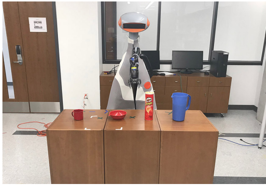
Fig. 5. Experimental setup with 4 YCB objects placed on a table between a person and a robot.
