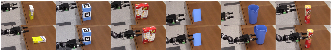
Figure 2: Affordances exhibited on our robot. The object/label pairs shown are: (a) sugar/tip (b) block/no-effect (c) crackers/push (d) prism/touch (e) pitcher/turn (f) chips/lean. The chips, crackers, and sugar objects are from the YCB [4] object set.
