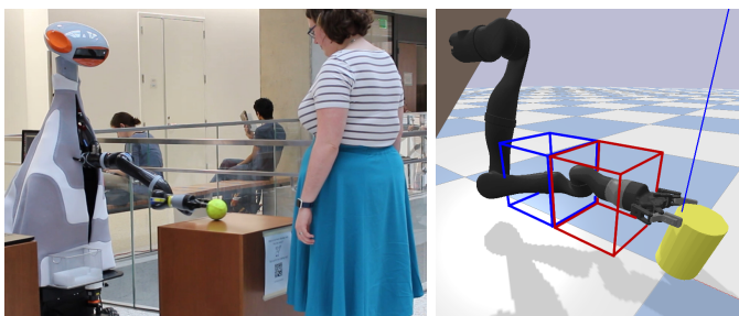
Figure 4: Left: our in-the-wild study recreated by one of the authors. The robot manipulates an object in a public area on campus and collects labels from passers-by. Right: a frame representative of the rendered simulation videos used in the online crowdsourced study. The object being manipulated is shown in yellow. Superimposed blue and red wireframes show the start and end positions of the robot’s wrist joint, respectively (for visualization only, not shown to participants).
